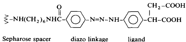
Scheme I. Affinity chromatography resin synthesized as described under Experimental procedures. The diazo linkage between the spacer and the ligand has been chosen for two main reasons: (1) the double bond makes the resin structure more rigid and prevents folding of the spacer; (2) there is a possibility of cleaving the ligand ( \pm bound protein) from the resin by using a reducing agent (e.g., dithionite).
